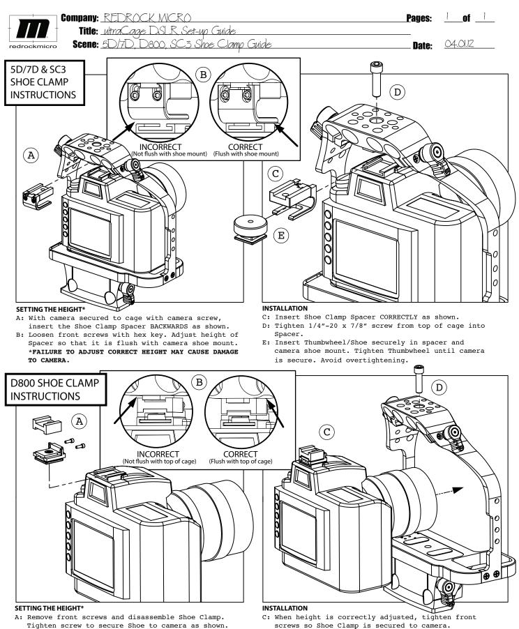
A: Remove front screws and disassemble snoe clamp.
