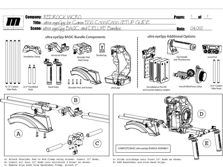
grip rods using screws. Replace blue knob.
