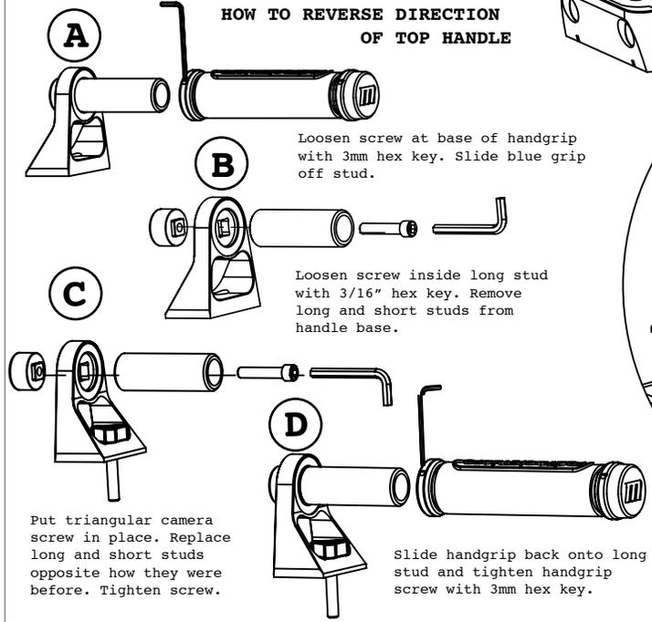
Loosen screw at base of handgrip with 3mm hex key. Slide blue grip off stud.
