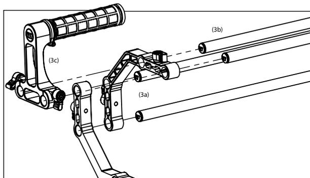
(3a) Insert 12in rods into 15mm arm
