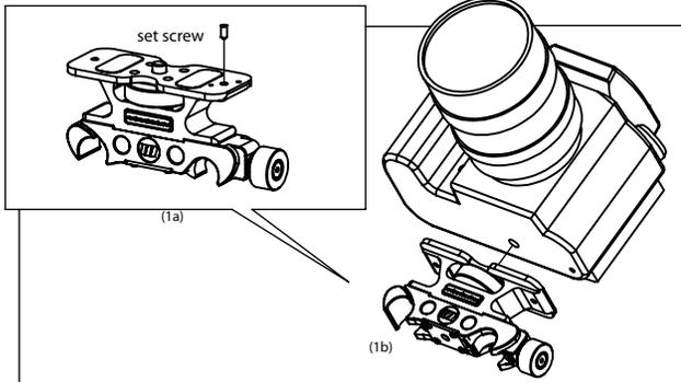
(1a) Add Camera specific set screw to DSLR Baseplate
