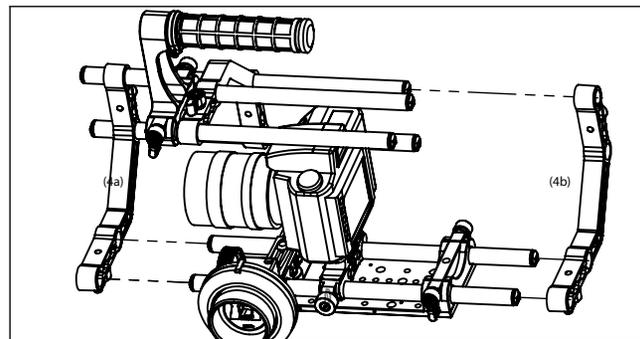
(4a) Attach Cage Build assembly to 12in Baseplate rods
