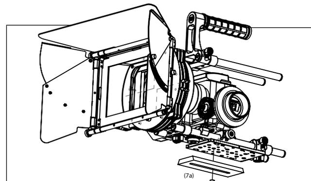
(7a) Attach quick release plate from your tripod to bottom of tripod plate
