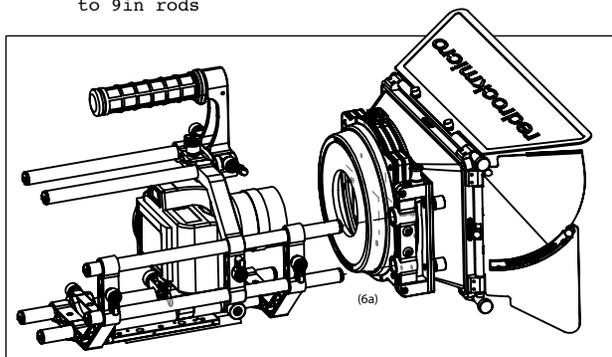
(6a) Attach microMatteBox directly to 12in rods
