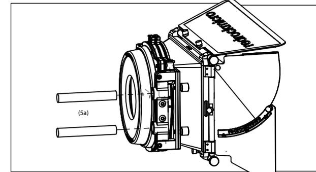
(5a) Remove 4in rods from the microMatteBox assembly
