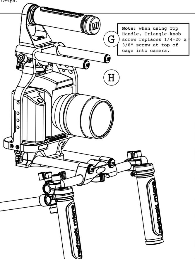
Note: when using Top Handle, Triangle knob screw replaces 1/4-20 x 3/8" screw at top of cage into camera.
