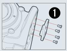
Remove supplied DoubleTap plate from ultraCage bottom. Remove standard mounting plate from camera bottom. Replace with DoubleTap as shown using Canon plate screws.
