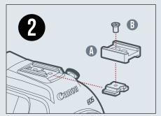
2. If required, attach Shoe Clamp Adapter (A) for C100 camera. Position clamp in camera shoe mount as shown and tighten screw (B).
