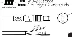
2 pin connector for use with Output 3. Do not attempt to mate with Outputs 1 and 2.
