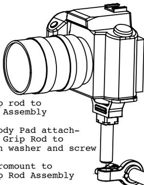
(2a) Attach Grip rod to Camera/Baseplate Assembly
