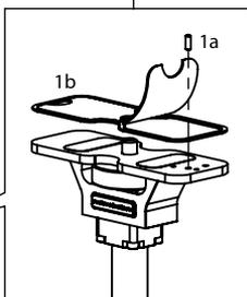
(1a) Attach camera specific set screw to DSLR Baseplate. Kit comes with Canon and Nikon set screws
