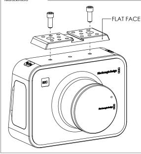
Align Top Plate with camera so the flat face is facing forward. Secure to camera with provided 1/4-20 screws.
