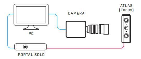
3. **Real-time performance capture of production crew** (such as CG movies where camera movement, lens control, etc. is all recorded for digital playback via Unreal or Unity game engines): in more advanced applications, Redrock UI controllers are used to stream real-time performance of the controller, such as pulling focus, changing zoom, adjusting camera pan/tilt, etc. these are addressable and behave nearly identical to lens control motors from an app development perspective
