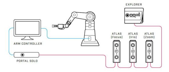
2. **Custom camera applications** that are driven by a computer application (such as advanced 3D and light field cameras): Custom PC applications can directly drive lens control motors in real time
